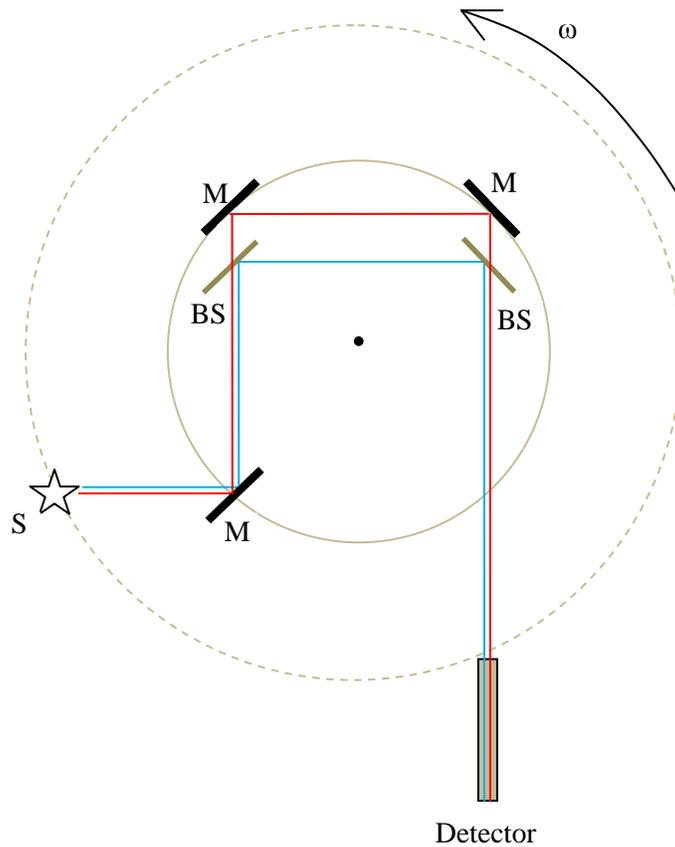
Here we propose a modified Sagnac experiment in which two light beams propagate in the same direction ( CW or CCW ), instead of in opposite directions, as shown above. M represents mirror and BS represents beam splitter.
