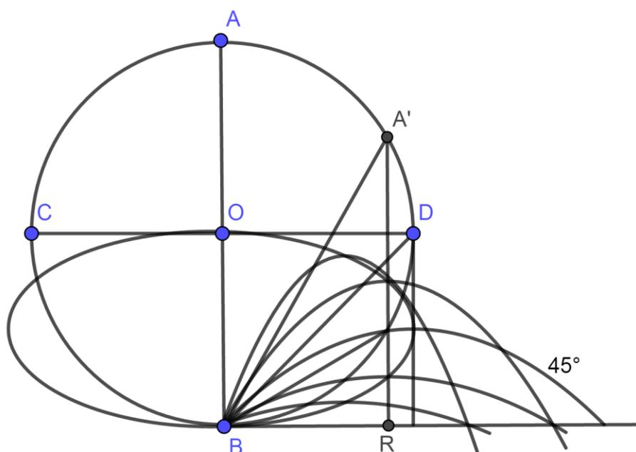
Fig. 3 The family of parabolic paths of projectiles shot from point B with constant speed  $v_B$  at different angles from the horizontal. The ellipse that passes through the apices of the parabolic paths is shown in the figure. This corresponds to the ellipse shown in reference 1.
