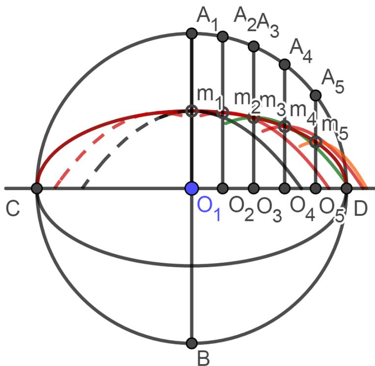
Fig. 2. Ellipse passing through the apexes of the parabolas
