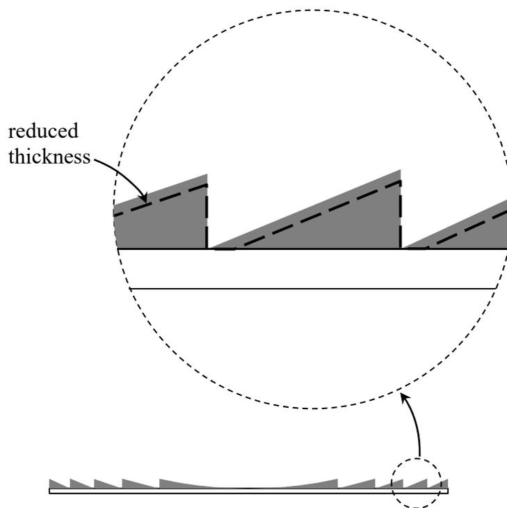
Figure 2. Cross-section of a sawtooth-profile phase-Fresnel lens (standard and thickness-reduced).
