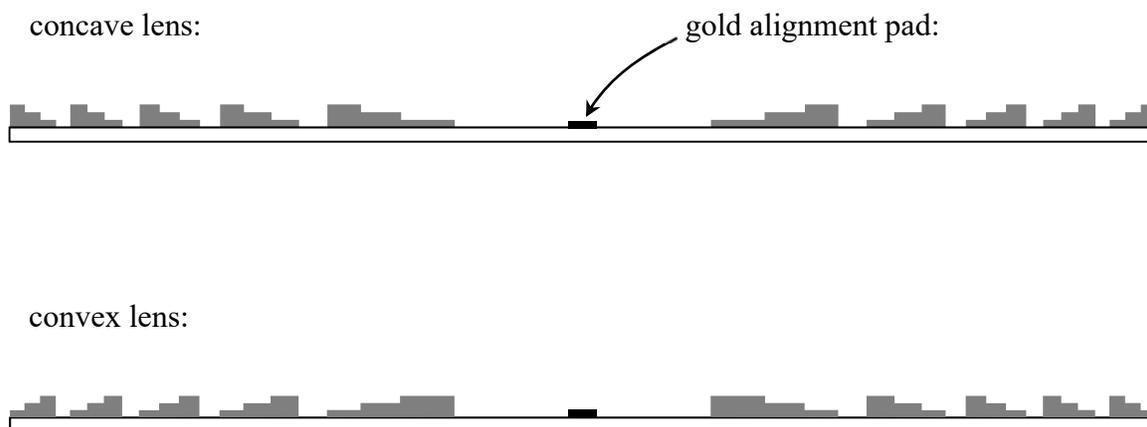
Figure 9. concave and convex lens forms with frontside alignment targets
