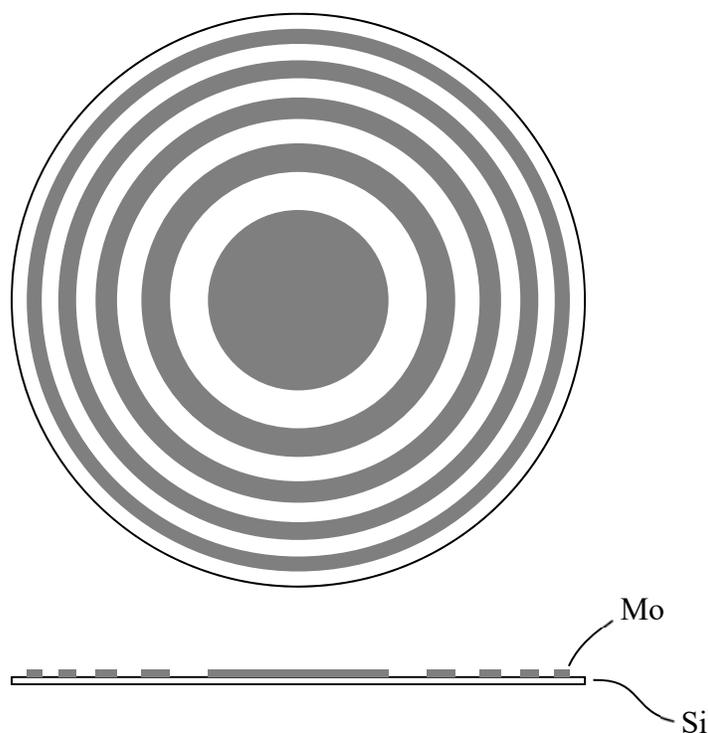
Figure 1. Plan view and cross-section of a zone-plate lens, which has a rectangular zone profile.
