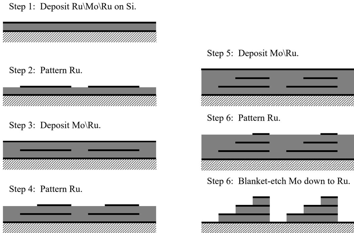
Figure 8. e-beam patterning steps for lens manufacture
