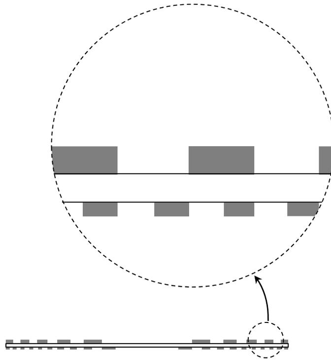
Figure 5. Double-sided EUV lens with zone-plate structures on both sides.
