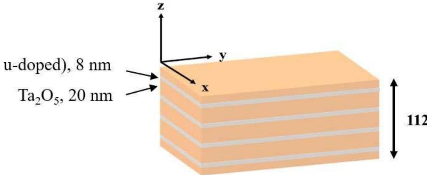
Cross-sectional view of the hyperbolic metamaterial examined in the new study shows layers of copper-doped silver and tantalum pentoxide. Credit: NIST
