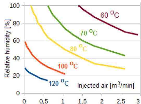
Fig. 2: The relative humidity of the exiting moist air as a function of the injected air volume (at 35 °C).
