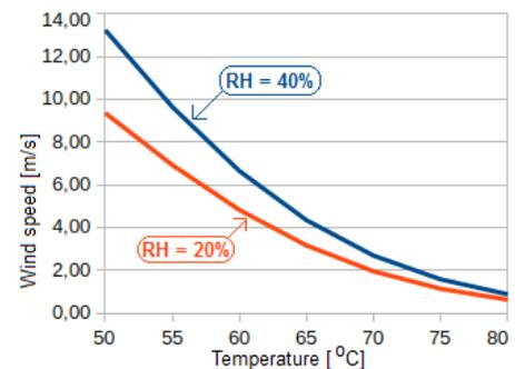
Fig. 1: Wind speed over a warm water surface to blow away the generated steam (30 kg/h).
