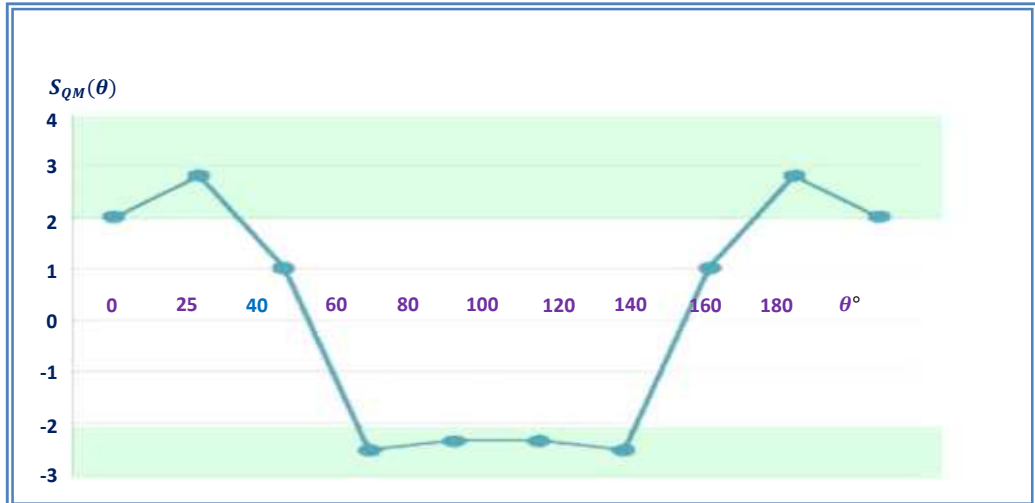
Fig 5: S_{QM}(\theta) , predicted by quantum mechanics for EPR-pairs. The conflict with Bell's inequalities occurs at |S| > 2 and it reaches a maximum for the set of orientations shown in Figure 4.
