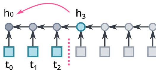
Miners can decrease or increase their cutoff at any time. In our example, the small-block miner could lower the cutoff from 2 to 1 by dropping every tree  $t_2$ , and storing  $h_2$ . Instead, to increase the cutoff from 2 to 4, the miner needs to download trees  $t_3 \dots t_4$ , and value  $h_3$ . The miner can authenticate appended trees and  $h$  value by hashing them, and comparing them against  $h_3$ .
