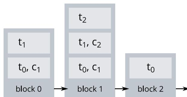
In addition to the tree with regular transaction  $t_y$ , each sub-block will include a tree with claims  $c_{y-}$ , as well as distinct drop values for the number of previous transaction trees, and previous claim trees. Big-block miners insert the transaction (moving a coin from  $y$  to  $y-1$ ) at height  $y$ , and include a claim that the recipient address has gained one coin at height
