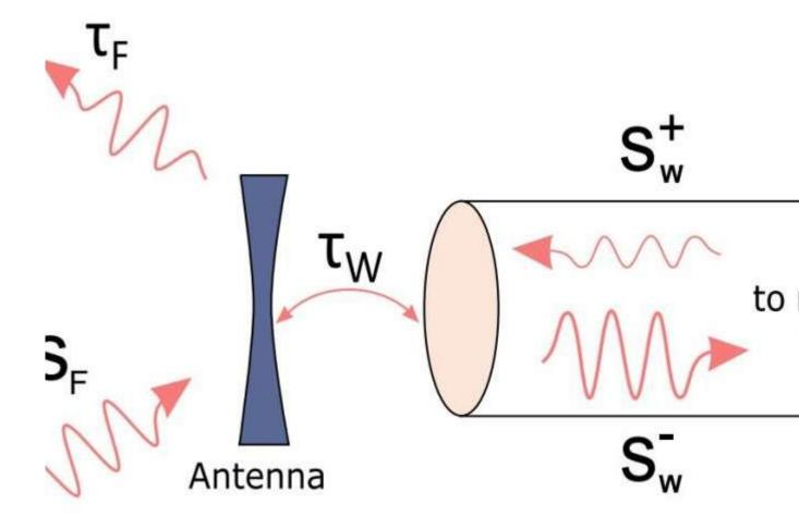
Receiving antenna. SF denotes incident radiation, while sw? is the energy that ultimately goes into the electrical circuit and sw+ is the auxiliary signal. Credit: Alex Krasnok et al./Physical Review Letters
