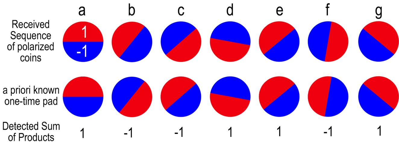
in the figure), then you can correctly decode the message, by simply performing a pixel-by-pixel multiplication of each received coin and the corresponding coin in the one-time pad, and sum all those product-pixels, to determine if the result is either positive (1) or negative (-1) as in the third line of the figure. (Red = +1, Blue = -1).
