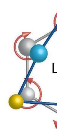
This diagram maps out atomic motion in separate phonon modes. At left ("LO" represents a longitudinal optical mode), selenium atoms exhibit a clockwise rotation while tungsten atoms stand still. At right ("LA" represents a longitudinal ...<u>more</u>
