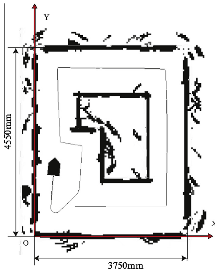
Fig. 9. Map building based on CFMW after improving the sonar model.
