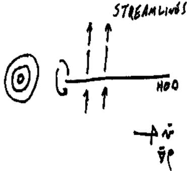
Figure 3: Diagram of the formation of a vortex at the trailing edge when the  $\vec{v}$  or  $\vec{\nabla}\rho$  is parallel to the hod surface.
