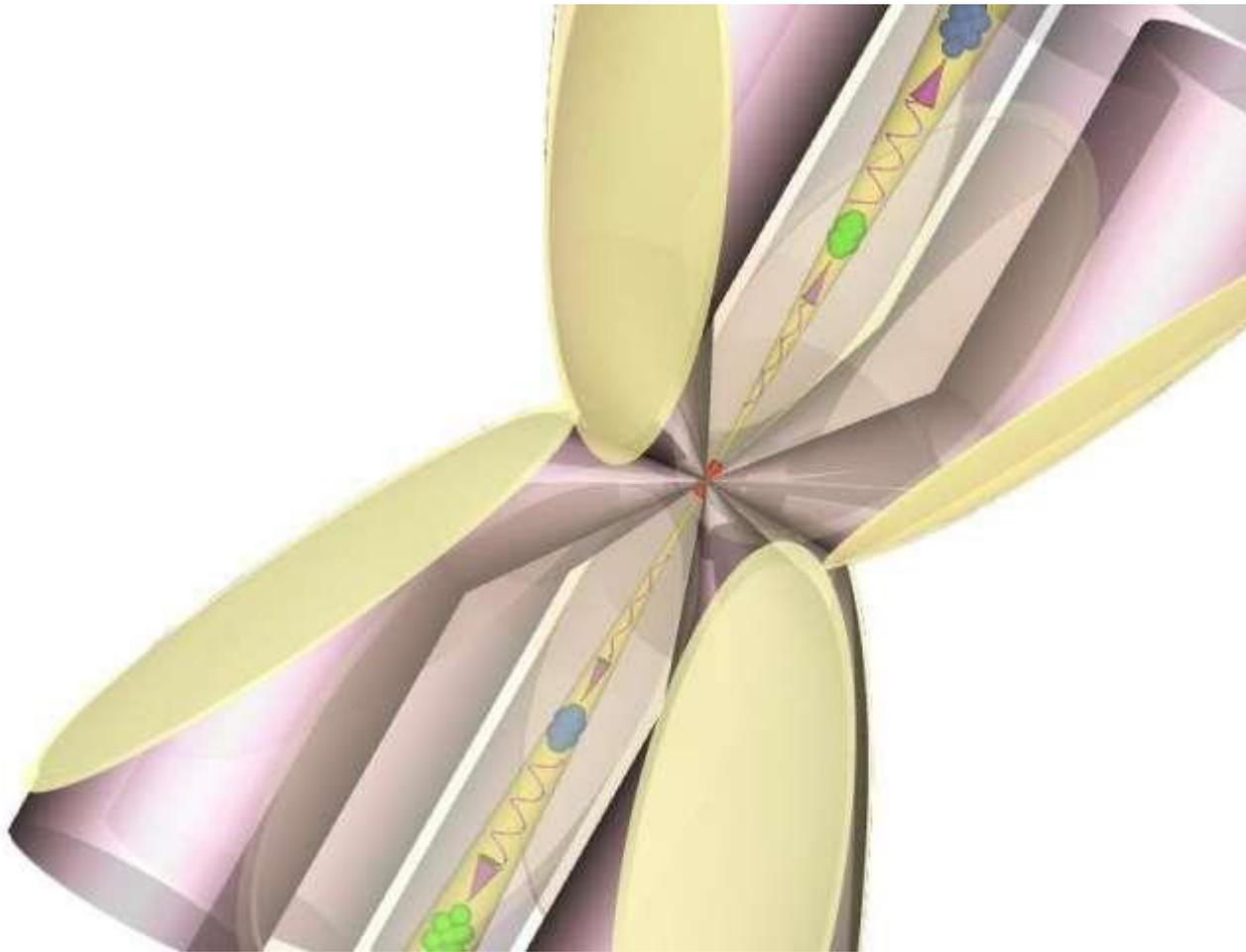
Electron and positron beams as well as gamma photons are emitted from the focus along the symmetry axis. Credit: E. Efimenko
