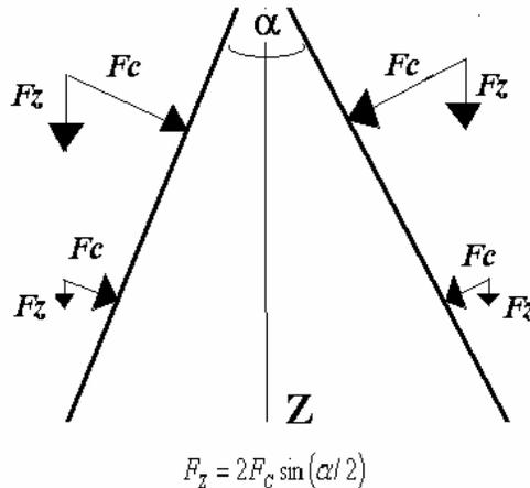
Fig.1. A projection of the force  $F_C$  onto Z axis develops an elemental thrust
