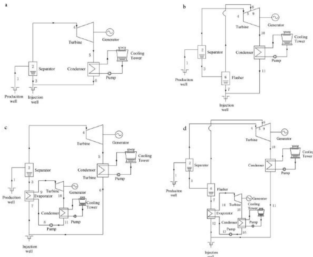
Fig.1. Schematic diagrams of four geothermal power generation systems
