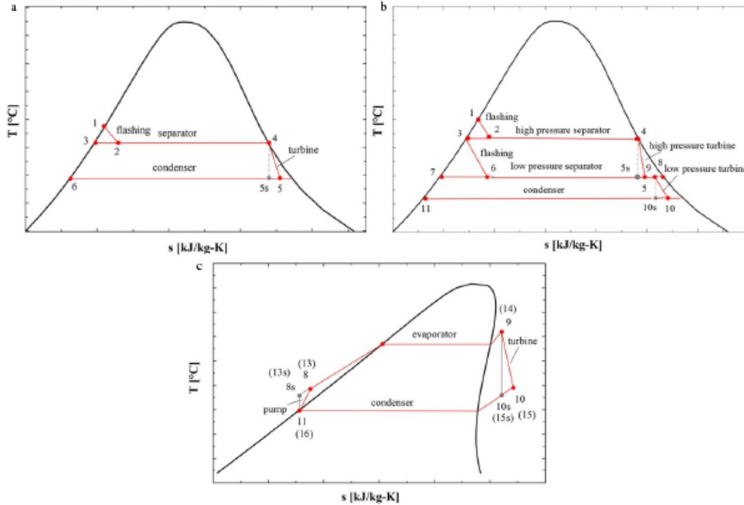
Fig.2. Temperature-Entropy diagrams of four power generation systems
