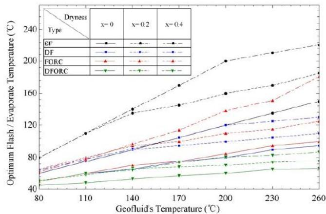
Fig.4. Optimum flash temperature of SF, 2nd-stage flash temperature of DF, and evaporation temperatures of FORC and DFORC under different geofluid's conditions ( $T= 80\sim 260\text{ }^{\circ}\text{C}$ ;  $x= 0, 0.2, 0.4$ )
