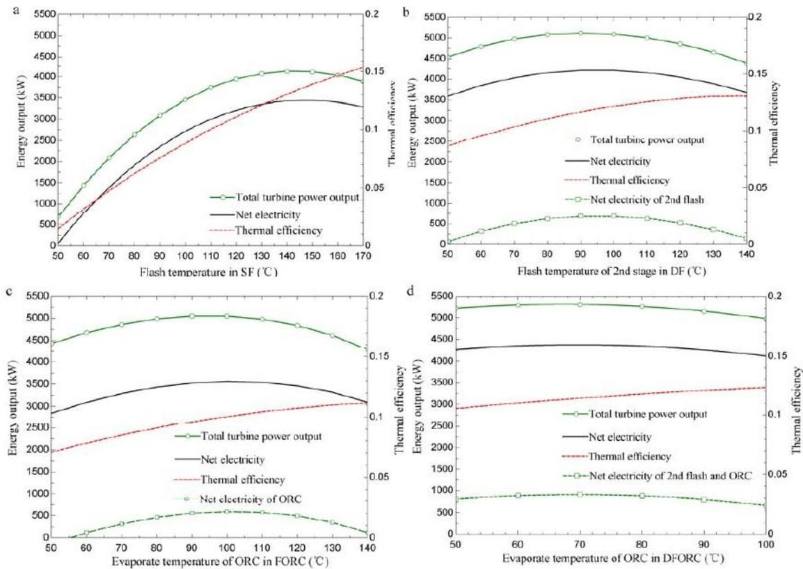
Fig.3. Calculation results for the optimization of flash or evaporation temperatures for four power generation systems in the given geofluid's condition ( $T=170^{\circ}\text{C}$ ;  $x=0.2$ )
