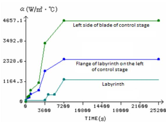
Figure 5. Variation curve of CHTC during low temperature startup
