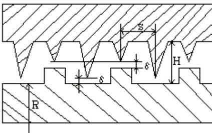
Figure 1. The geometry of labyrinth<sup>[4, 5]</sup>
