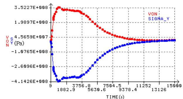
Figure 10. Equivalent stress and axial stress at the flange of labyrinth during high temperature startup
