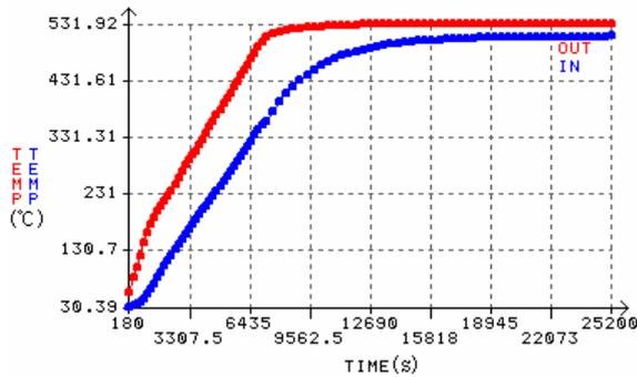
Figure 7. Temperature behavior in the inside and outside of rotor during the low temperature startup
