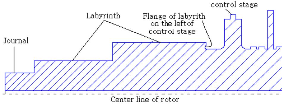
Figure 2. The geometry of a 50Mw turbine rotor in “S” power station
