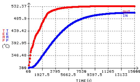
Figure 9. Temperature variation curve at the flange and in the inside of rotor during high temperature startup
