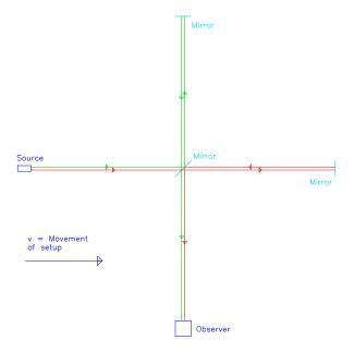
Fig. 16: Schematic setup of the Michelson/Morley experiment
