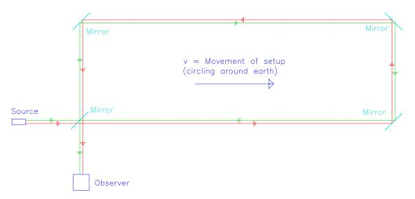
Fig. 15: Schematic setup of the Michelson/Gale/Pearson experiment
