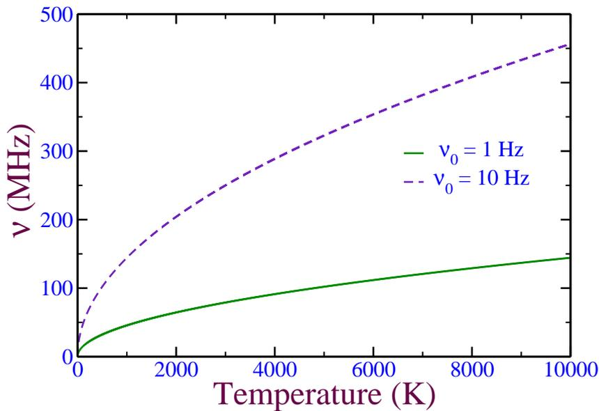
Figure 1: Variation of emission frequency ( $\nu$ ) with heating temperature ( $T$ )
