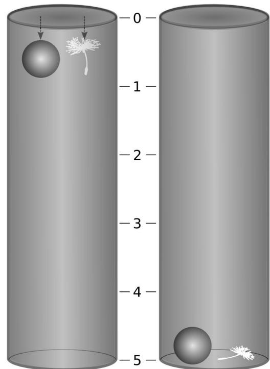
Figure 1: Free Fall in Vacuum Chamber
