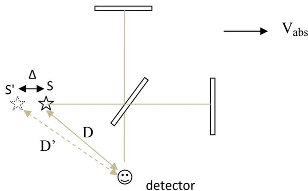
From the above diagram of the Michelson-Morley experiment, we see that the effect of absolute velocity is just to create an *apparent* change of the position of the light source *as seen by the detector*. The apparent change in position is determined by the direct source-detector distance  $D$ , the orientation of the source-detector line with respect to the absolute velocity and the magnitude of the absolute velocity [2].
