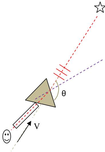
The Airy experiment is shown below, in which the star is observed through a telescope filled with water.
