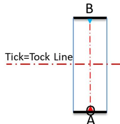
The measurement comes with a delay between a flash and its observation which depends on the distance between the observer and the source of the flash at A or B.
