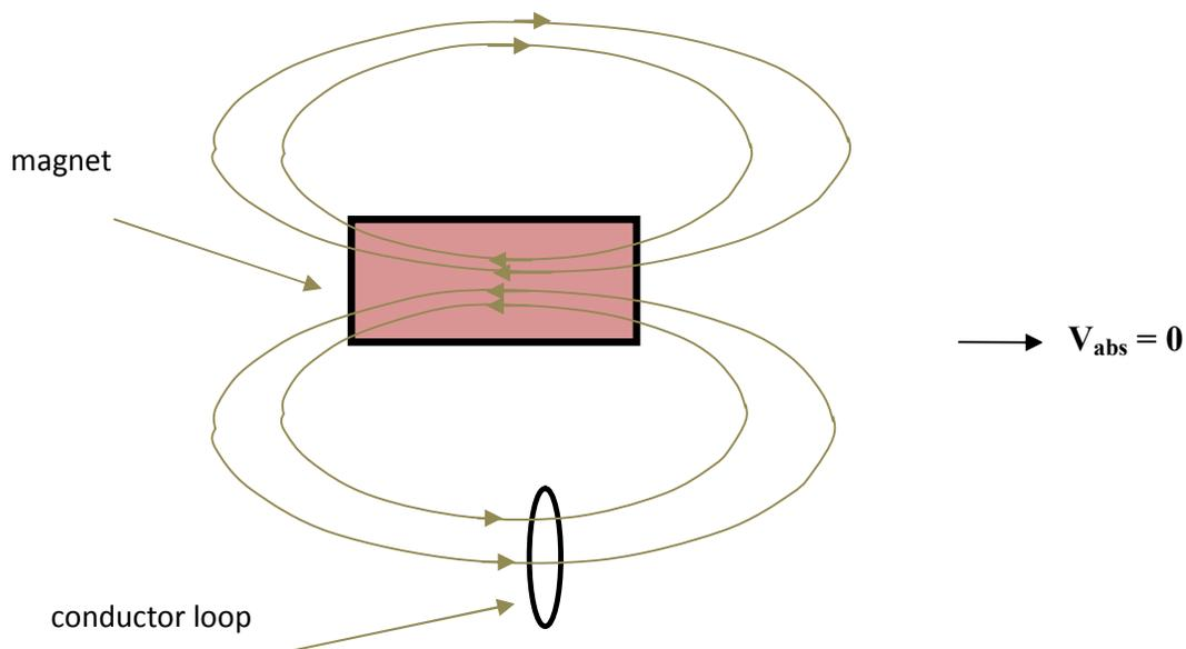
*Current will not be induced in the conductor for any position of the conductor relative to the magnet if they are both at absolute rest and hence at rest relative to each other.*
