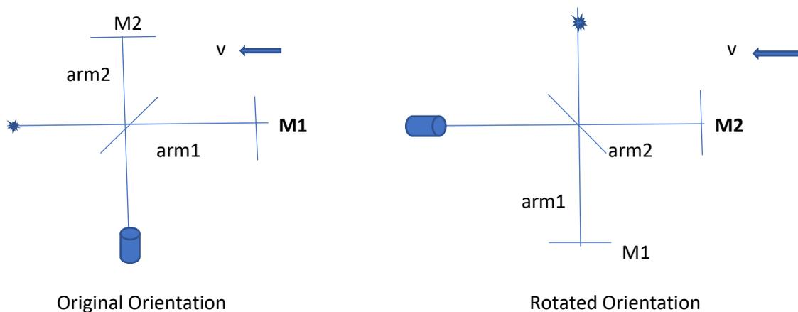
Looking at the experiment from the point of view of the wave theory of light, we can see that the two beams of light have the same situations in both the original and rotated positions of the apparatus. In both situations one arm is parallel to the direction of the earth’s motion and the other is perpendicular
