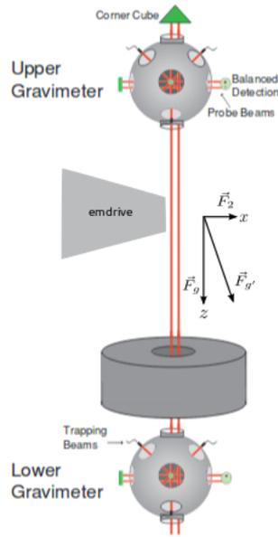
**Fig. 4** Cesium interferometer based gravity gradiometer. Hyperfine splitting of cesium in its ground state acts as the ruler of the apparatus which employs a  $\pi/2 - \pi - \pi/2$  light pulse sequence on two identical ensembles of cesium atoms. This apparatus achieved a differential acceleration sensitivity of  $4 \times 10^{-9} g / \sqrt{Hz}$  and an accuracy of  $\leq 10^{-9} g$  [83].
