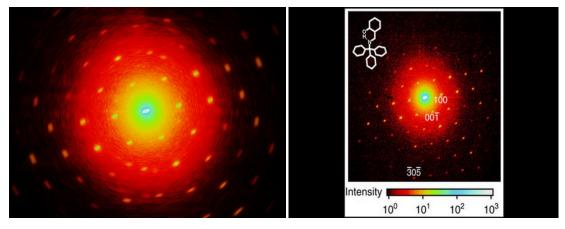
If ultrashort electron pulses hit a bimolecular crystal, they are diffracted from it. As a result, one obtains a characteristic diffraction image of the atomic structure. Credit: Graphic: Alexander Gliserin [4][5]
