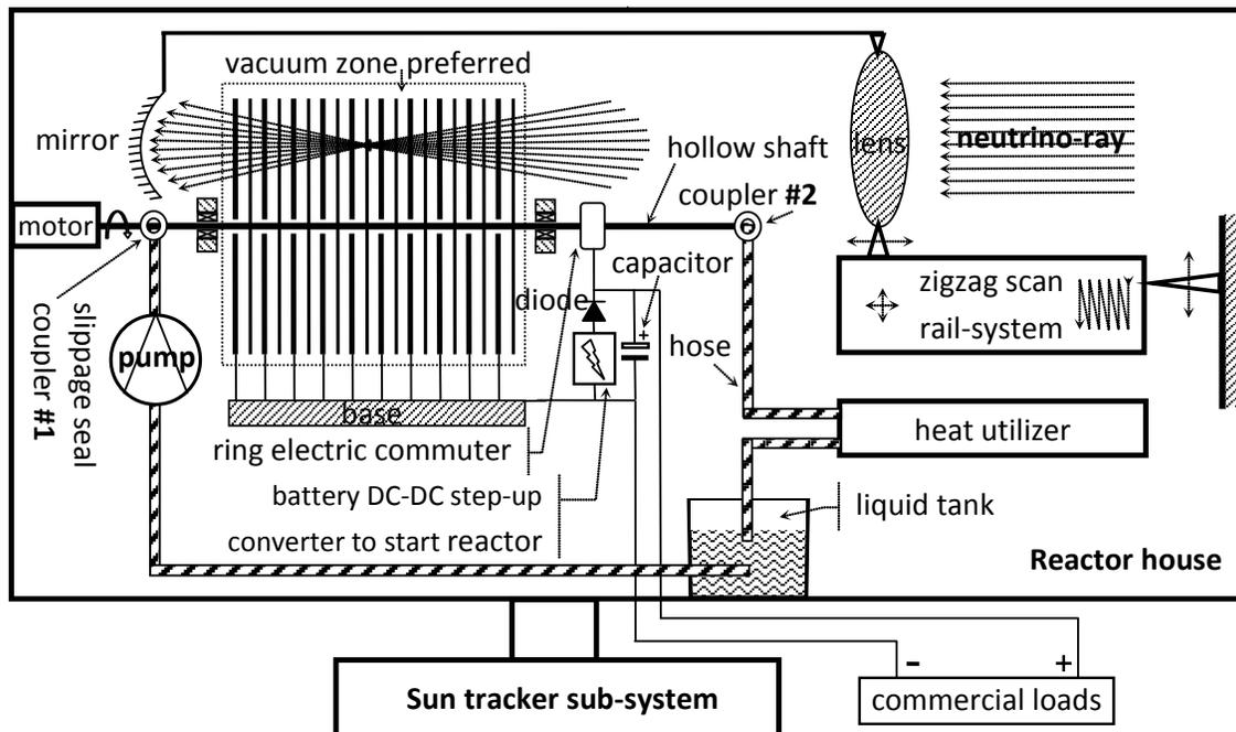
The starter comprises battery and step-up high voltage DC-DC converter, and is switched off after stable state is established, then is recharged by output in float mode.
