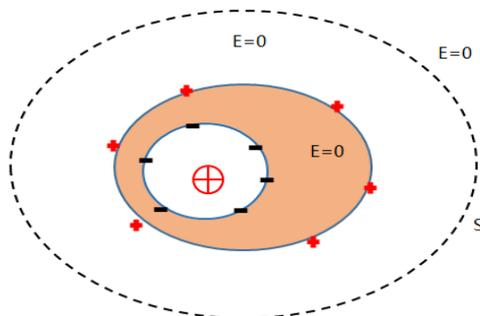
**Figure2.** A closed surface S enclosing the whole conductor. The net electric flux through the closed surface is zero, due to the electric field is zero everywhere outside the conductor.
