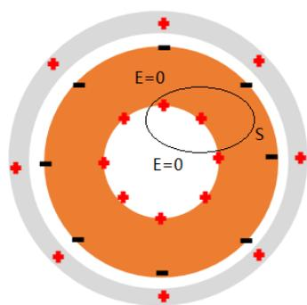
**Figure5.** A spherical electric charge layer encloses a conductor cavity. A closed surface  $S$  contains two parts. One part is in the cavity and the other inside the body of the conductor.
