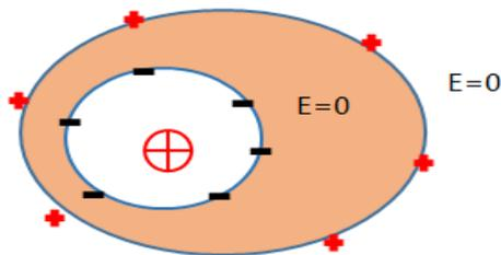
**Figure1.** A neutral conductor cavity containing a positive electric charge. Under electrostatic equilibrium state, the electric field is zero inside the body area of the conductor and in the area outside the conductor.
