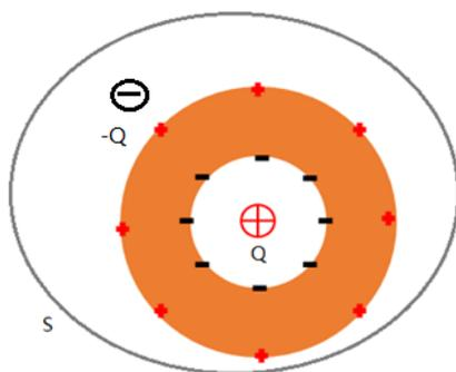
**Figure4.** A neutral conductor cavity enclosing a positive electric charge  $Q$  and there is another negative electric charge  $-Q$  in the vicinity of the conductor.  $S$  is a closed surface enclosing the whole system.
