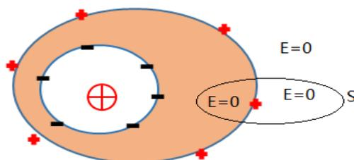
**Figure3.** A closed surface S consists of two parts. One part is within the body of the conductor and the other outside the conductor.
