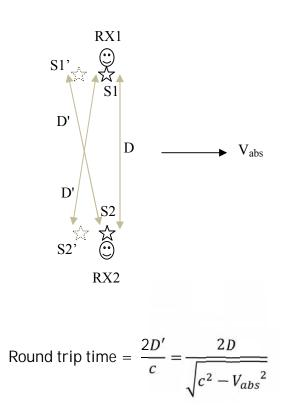
We see that the round trip time and hence the clock rate is affected by absolute velocity. The higher the absolute velocity, the slower the clock. Only the rate of the clock slows down ; there is no 'time dilation'.
