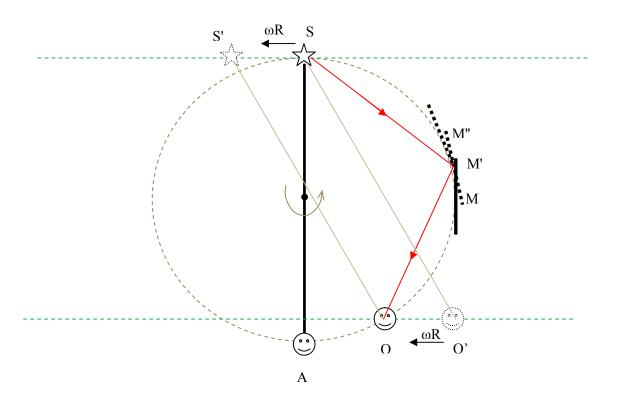
The problem is to determine the time delay of light between emission from the source S and detection by the moving observer A, after reflection from the mirror.
