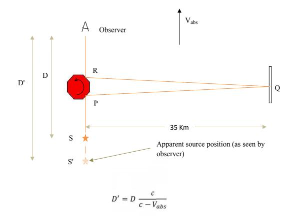
To clarify this interpretation, assume that sensors are put at points P, Q and R. Points P and R are points in space where the light is reflected from the rotating mirror, point Q is point on the distant mirror where the light is reflected. If a short light pulse is emitted by the source at time t = 0, then the light will be detected at points P, Q, and R, at times  $t_P$ ,  $t_Q$  and  $t_R$ , respectively.
