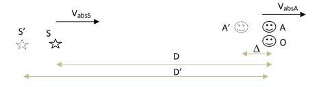
Suppose that the distance between a co-moving observer O ( the absolute velocity of O is the same as the absolute velocity of the source,  $V_{absS}$ ) and the source is D and that the moving observer (A) was at point A' relative to the source at the instant of light emission. Suppose that observer A is just passing through point A ( the same as point O ) at the instant that observer O detects the light. Therefore, observer A will also detect the light at that instant.
