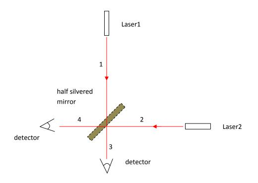
Consider the lasers to be ideal : their coherence time is infinite , and both have exactly the same frequencies and intensities, the arm lengths are exactly equal. The beam divergences are nearly zero.
