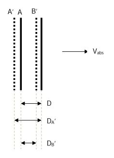
$D_A'$  is the apparent distance of plate A as seen by plate B.  $D_B'$  is the apparent distance of plate B as seen by plate A. Strict application of AST shows that, to a point charge on one capacitor plate the opposite plate is not a plane but somewhat curved. However, we can use the above simplistic assumption to a good approximation.
