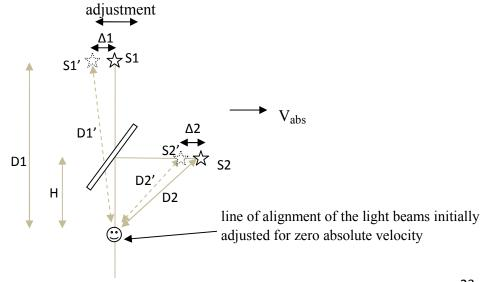
With zero absolute velocity, the two light beams arriving at the detector are adjusted to be aligned. Then, due to non zero absolute velocity, the two beams will be misaligned and a fringe shift will occur. The position of the source S1 may be adjusted (towards the right) until the two light beams are aligned again. The amount of adjustment of position of S1 required to align the two beams again can be used to determine the absolute velocity.
