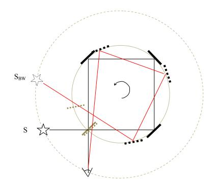
The position of the source apparently shifts towards when looking in the forward direction and away from the detector when looking in the backward direction. Therefore, a difference between path lengths of the backward light beam and the forward light beam arises resulting in a fringe shift. The apparent sources are at rest relative to the observer ( because the real source is at rest relative to the observer ) and the speed of light is constant relative to the apparent source.
