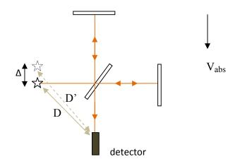
What is the effect of absolute velocity in this case? In the same way as above, we ask: what is the effect of actually, physically shifting the source position from S to S'? In this case also there may be a very small fringe shift because the two beams will be misaligned and will have slightly different path lengths. This may be why a very small fringe shift was always observed in conventional MM experiments.
