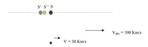
The sun will now appear to be at position S"(20 arcseconds ahead of S'), due to earth's *relative* motion. However, this does not mean that the light rays are coming from the direction of S"; it is
