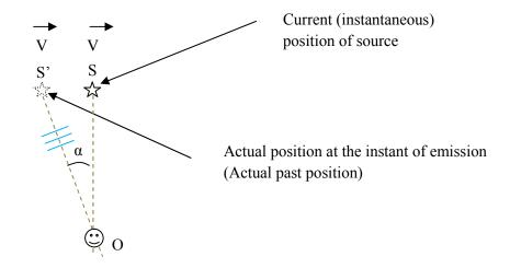
The source position now (at the moment of observation) is at S, moving with velocity V. But the source was at position S' at the moment of emission, moving with velocity V also, assuming uniform motion.
