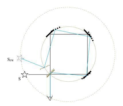
The apparent source  $S_{FW}$  and the apparent position of the mirrors as seen by the detector have been shown above, along with the real, instantaneous position of the mirrors and the source drawn with solid lines. We can see that the path length of the light will be apparently reduced in the forward direction due to rotation of the apparatus.
