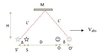
The time T elapsed for the light to travel from S', reflect at mirror, then arrive at O' is equal to the time taken for the observer to move from O to O'. The speed of light is c relative to the apparent source. We have to determine the speed of light c' in the dashed light ray, as seen in the absolute reference frame.
