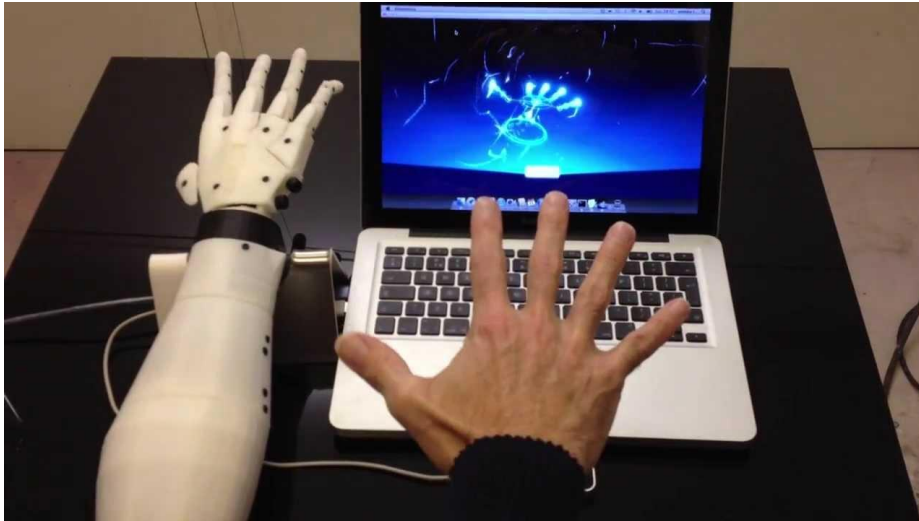
Figure 7. Gesture Control using Leap Motion device [1].
