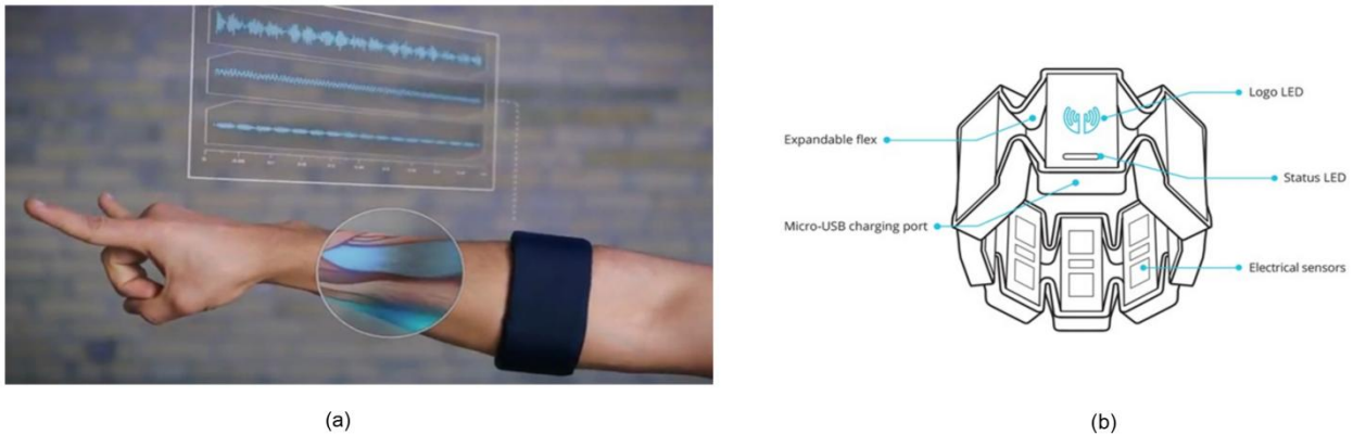
Figure 3. (a) MYO Armband reading electrical signals from muscles. Source: MYO. (b) Structure of MYO Armband. Source: MYO.
