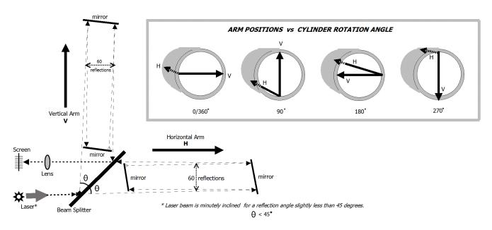
**Figure 1**: Schematics of the modified Michelson Interferometer and its mounting in the cylindrical frame. For simplicity, some components are omitted and distances/angles may not be in correct scale.
