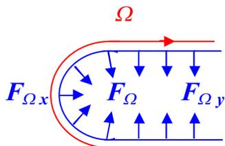
Near the edges of the upper side of the ring, a gyrotation force is acting due to the velocity of the edge's part and its mass, given by equation (1.1).
