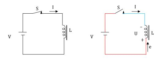
Let us consider the inductor circuit again by using a current source, as shown in the next figure, to further clarify the idea. Suppose that the current I is initially zero and then continuously increased at some rate. This means that the current source is *forcing* current through the circuit, with the electron flow as shown.
