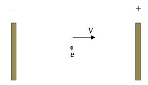
Suppose that the electron is initially moving with some constant velocity V. This can be done by initially switching on the voltage across the plates briefly and switching it off, discharging the plates so that the electric field will be zero. With zero electric field, the electron will continue moving with a constant velocity.
