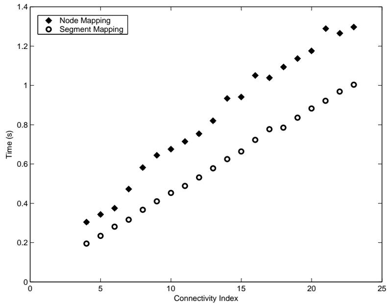
Figure 6: Execution time in seconds versus the average connectivity index of the network for the node mapping and segment mapping algorithms. All networks used in these tests have a single section with five million nodes.
