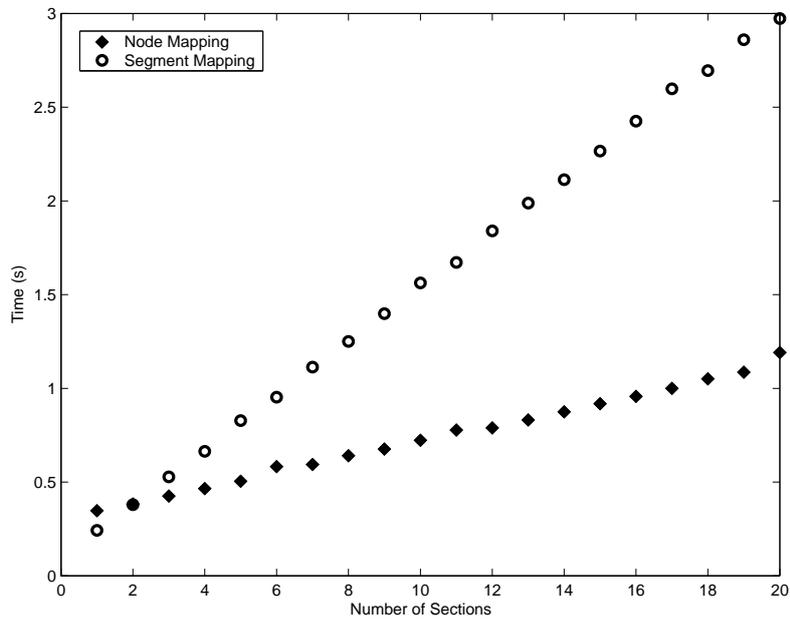
Figure 7: Execution time in seconds versus the number of network sections for the node mapping and segment mapping algorithms. All networks used in these tests have about five million nodes with an average connectivity index of approximately 5.
