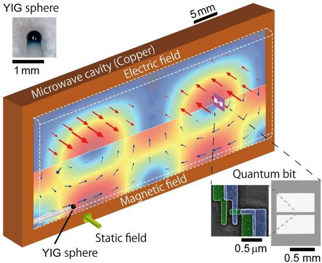
Illustration of magnet-qubit coupled system A magnet (yttrium iron garnet; YIG) and a superconducting qubit are placed with a separation of 4 cm. The electric field in the cavity interacts with the qubit, while the magnetic field interacts with the magnet. At an extremely low temperature of around -273 degrees centigrade, magnons, i.e., quanta of the fluctuations in the magnet, coherently couple with the qubit through the electromagnetic field of the cavity.
