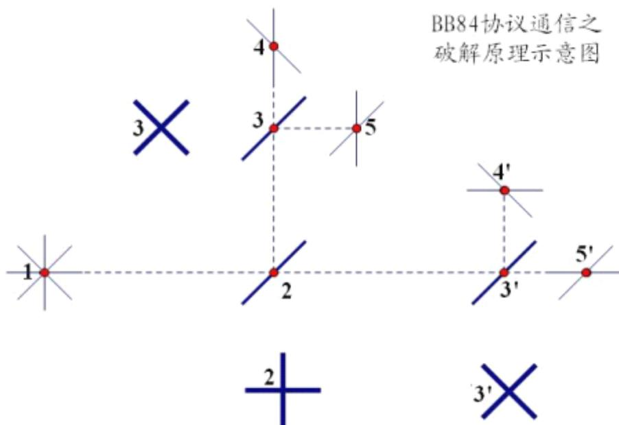
As shown in the figure, 1 is a single-photon with polarization state encoded by the listener and has 4 possible states of polarization. After passing through the first-order
