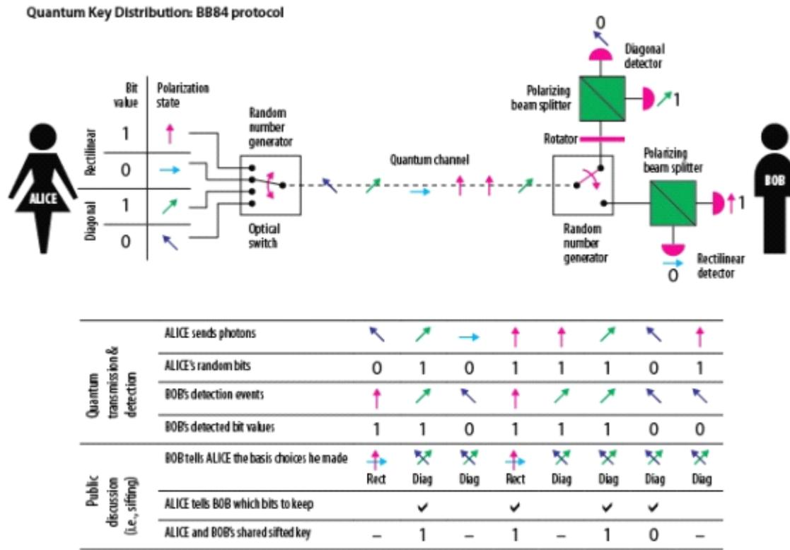
In the figure, the green square of Bob represents the PBS, which is the "polarizing beam splitter" mentioned above. Its basic function is to divide two linearly polarized photons whose polarization states are orthogonal to each other - to two different (Dd) as represented by the purple semilunar icon in the picture; if Bob uses the wrong analyzer (the light path switch identified as RNG in the figure to toggle in the wrong state), as shown in the figure, the photodetector (Dd) In the
