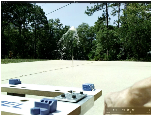
Figure-1, Sphere-cone riding on blast of water
