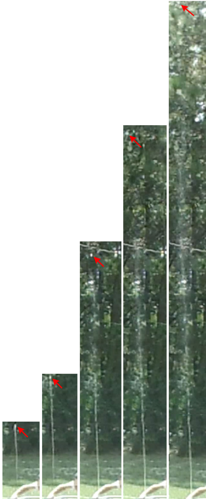
Figure-7, Sequence of movie images taken during external-jet propelled flight (0.15 to 1.19 sec). See measured (V, Z) and theoretical (V, Z) in TABLE-1 then plotted (V, Z) in Figure-8 and Figure-9.
