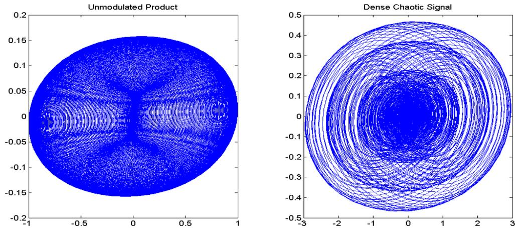
From the phase portraits, one can see the rich patterns in the engineer's chaos, and thus its capacity to hold information in the phase space. One can also see how modulating the carrier signals before multiplying them changes its nature, to provide the phase portrait of the dense chaotic signal.
