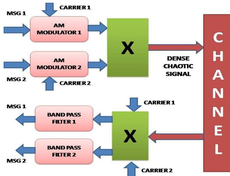
The dense communication is achieved by modulating the sinusoids of ' $f$ ' and ' $rf$ ' before multiplying them to generate chaos. These AM modulated signals are shown below:
