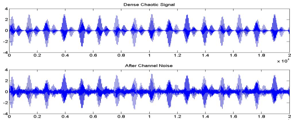
At the receiver end, the dense chaotic signal is fed to a multiplier, which multiplies the incoming signal by the product of the carrier signals generated locally. Following this, band pass filters with suitable specifications are used to extract the two message signals from the composite signal. The generated signals are shown as follows, compared with the transmitted messages both in time waveform and frequency spectrum:
