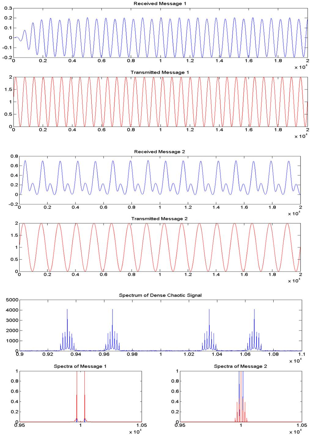
It is seen that one is able to successfully demodulate the message signals with reasonable amount of accuracy, even in spite of the 18dB channel noise.
