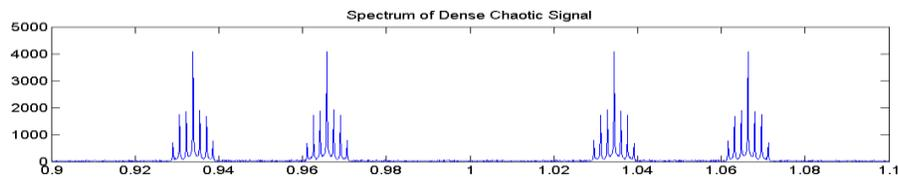
This dense chaotic signal thus forms the composite signal, and is the one transmitted through the channel. The channel is represented as Additive White Gaussian Noise (AWGN) with a nominal Signal-to-Noise Ratio (SNR) of 18dB [6]. The signals before and after adding noise are shown below:
