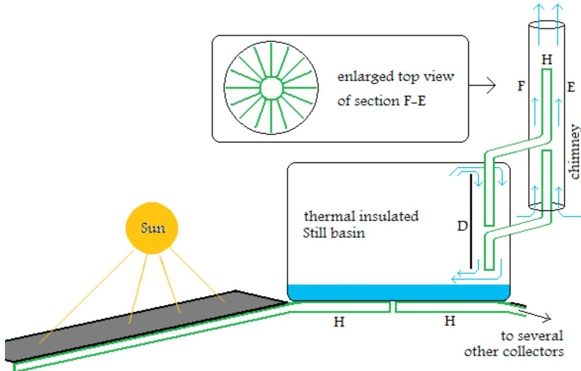
The picture shows how these demands can be realized technically. The heat energy of several solar collectors is transported via heat pipes (H) to a significantly smaller distillation vessel with good thermal insulation. This concentration is a way to raise the water temperature.
