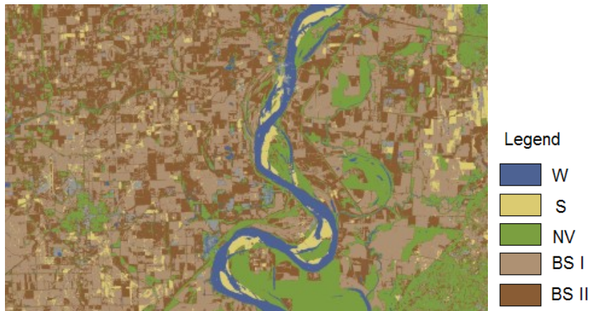
Figure 10: Classified image. Land cover types are Water (W), Sand (S), Native Vegetation (NV), Light Bare Soil (BS I) and Dark Bare Soil (BS II).
