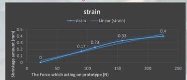
we found direct proportional between the force acting on prototype and strain
