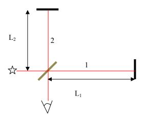
According to Lorentz contraction theory the time it takes light to traverse back-and-forth along the Lorentz – contracted length of the longitudinal arm is given by:
