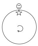
Assume that the light source emits light in the opposite directions tangentially. The two light beams travel in circular paths in opposite directions before being detected at the detector. A circular mirror is used to make light travel in circular path.
