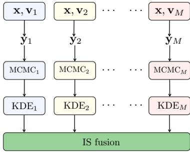
Figure 2. Graphical representation of Parallel Marginal Markov Importance Sampling scheme:  $M$  local MCMC chains are run, each one addressing one partial posterior  $\bar{\pi}_m$ . A kernel density estimation (KDE) for approximating the marginal partial posteriors  $g_m(\mathbf{x}|\mathbf{y}_m)$  is performed locally. Then, an importance sampling fusion is employed for providing a global estimator of the global parameter  $\mathbf{x}$ .
