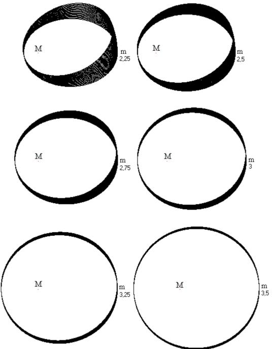
The following pictures show how to develop a rosette trajectory. The initial distance between bodies  $\mathbf{M}$  and  $\mathbf{m}$  in each successive exercise has the same value:  $\mathbf{Mm}=6$  l.u. (length units). But with increasing
