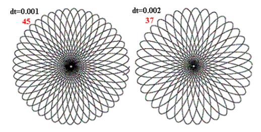
It can be seen that reducing the size of dt by half (from dt=0.002 to dt=0.001) results in that the number of rosette leaves increased from 37 to 45 leaves. In contrast, the figure below shows the difference in images of trajectories, where the value dt is even smaller - because dt=0.00025 and dt=0.000125. In this case when the value of dt is reduced by half the number of leaves remains approximately unchanged.
