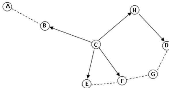
**Fig. 11.** Node 'C' broadcasts its new route to Node 'D'
