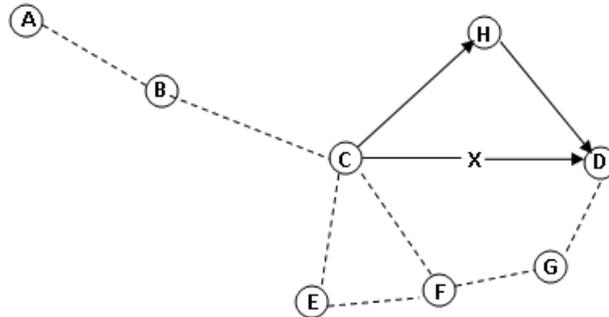
**Fig. 10.** Node 'C' reconstructs its route to Node 'D'
