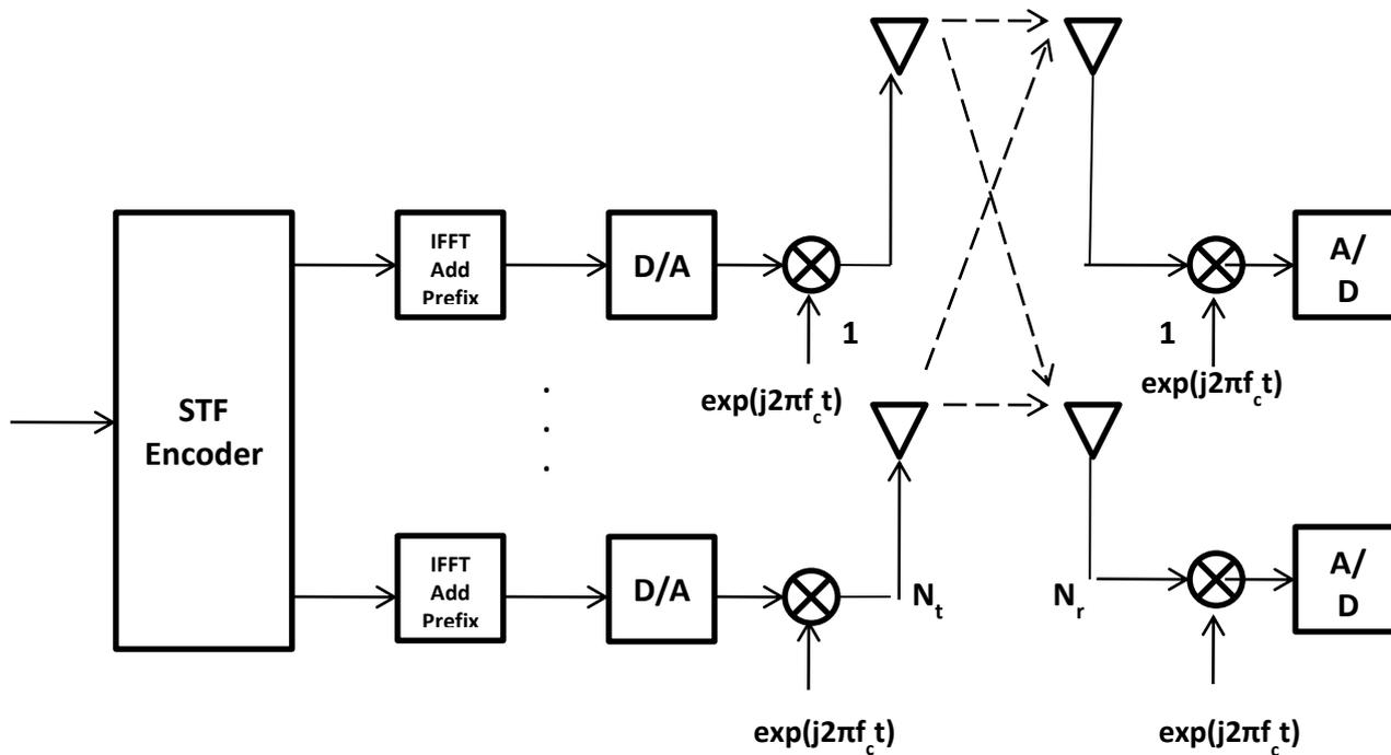
Figure 1 MIMO-OFDM multiband UWB system
