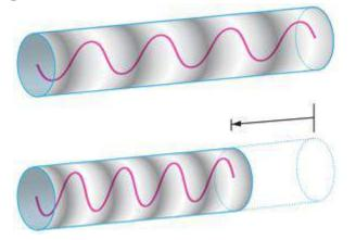
**Figure 1:** A resonator for the dynamical Casimir effect. The initial length of the resonator is shown in the upper illustration. The sine wave represents one of the modes of the resonator, initially populated by vacuum fluctuations. The length of the resonator is suddenly changed (lower illustration). The wavelength and frequency of the sinusoidal mode changes rapidly. The change is nonadiabatic, so the vacuum fluctuations are amplified, creating real photons.
