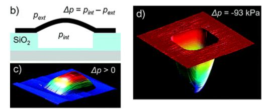
"We demonstrate that a monolayer graphene membrane is impermeable to standard gases including helium. By applying a pressure difference across the membrane, we measure both the elastic constants and the mass of a single layer of graphene. This pressurized graphene membrane is the world's thinnest balloon and provides a unique separation barrier between 2 distinct regions that is only one atom thick."
