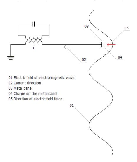
From the figure 1 and 2, we can see that the direction of electric field force can keep the same if the charge on the metal panel synchronizes with the electromagnetic wave. Because the direction of electric field force on the metal panel does not change, so the thruster will do directional movement.
