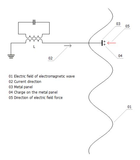
Figure 2: The Right Half of the Electromagnetic Wave Cycle.
