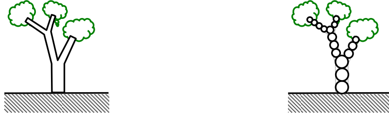
Figure 1. A two-dimension tree model: solid beam model (left) and granular particle interactions model (right).
