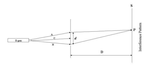
**Fig.1. Schematic diagram for the double slit experiment with electrons:** An electron gun shoots mono-energetic electrons at the double slit (width *d*) arrangement. Three electron trajectories 'A,' 'B' and 'C' are shown for illustration. Trajectory 'A' passes through upper slit, trajectory 'B' passes through lower slit and trajectory 'C' hits the barrier in between the double slit. The screen S records the interference pattern from electrons passing through the double slits.
