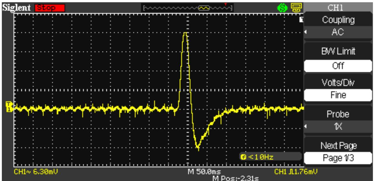
Fig. 8. Shape of pulse with the rapid withdrawal of the model of the charged amber from Faraday's cage.
