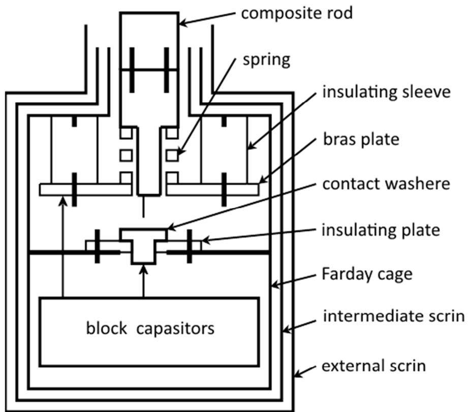
Fig. 4. The schematic of experimental installation.
