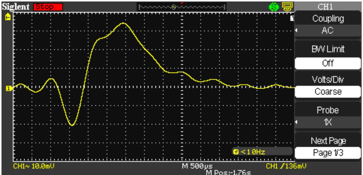
Fig. 15. Form of the voltage pulse between the external screen and the screen of Faraday’s cage, obtained with capacitor discharge with a capacity  $6000 \mu F$ , charged to the stress  $300 V$ . Scale along the X-axis is  $5 ms$ .
