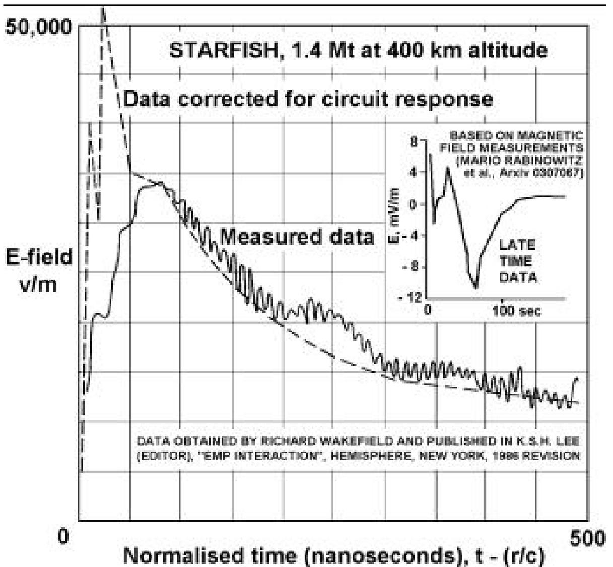
Fig. 1. Experimental dependence of amplitude EMP on the time, obtained with the tests according to the program “Starfish”.
