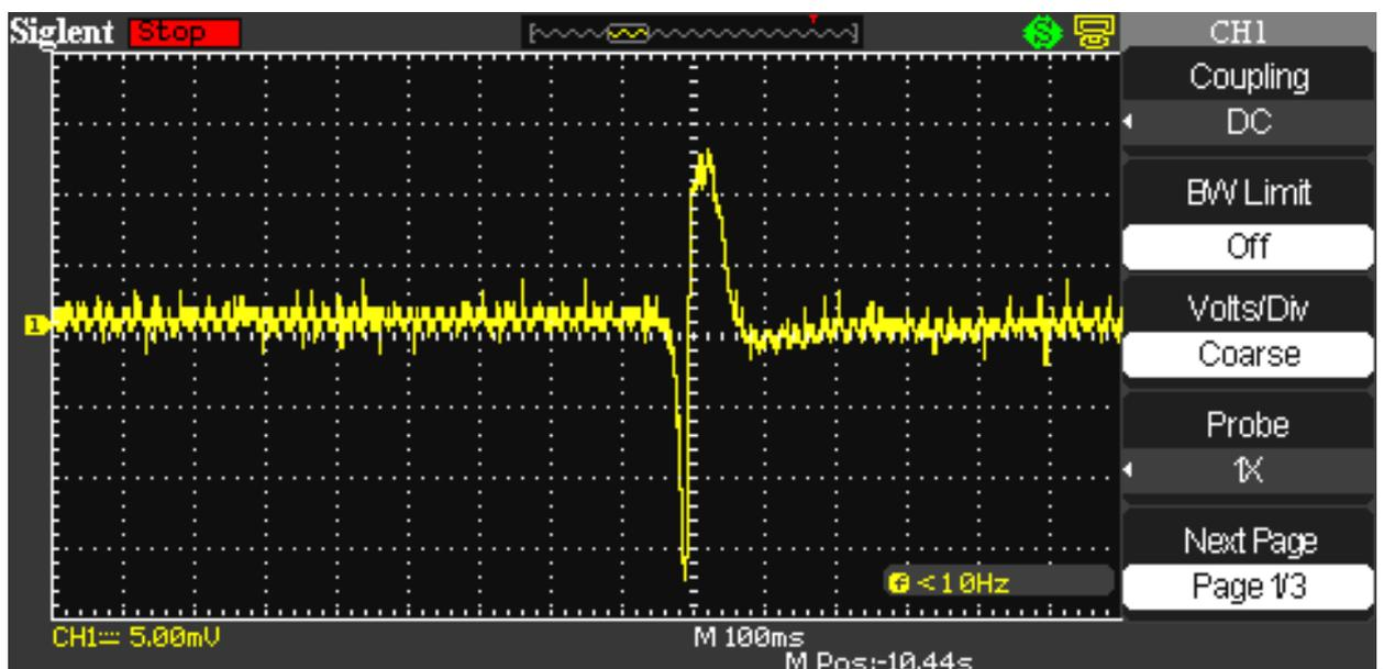
Fig. 7. Shape of pulse with the rapid withdrawal of the model of the charged amber from the Faraday's cage.
