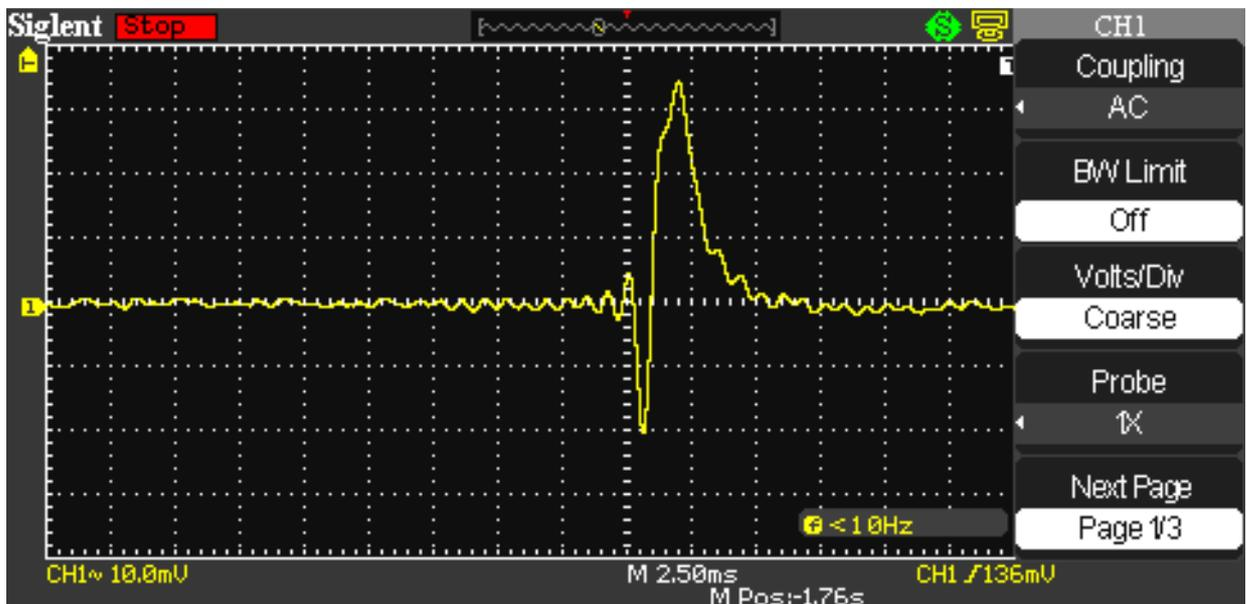
Fig. 14. Form of the voltage pulse between the external screen and the screen of Faraday's cage, obtained with capacitor discharge with a capacity  $6000 \mu\text{F}$ , charged to the stress 300 V. Scale along the X-axis is 5 ms.
