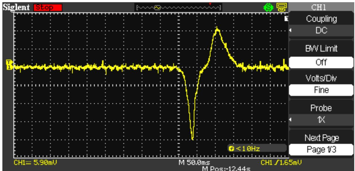
Fig. 9. Voltage pulse, obtained with the rapid introduction and the subsequent withdrawal from the Faraday's cage of the charged model of amber.
